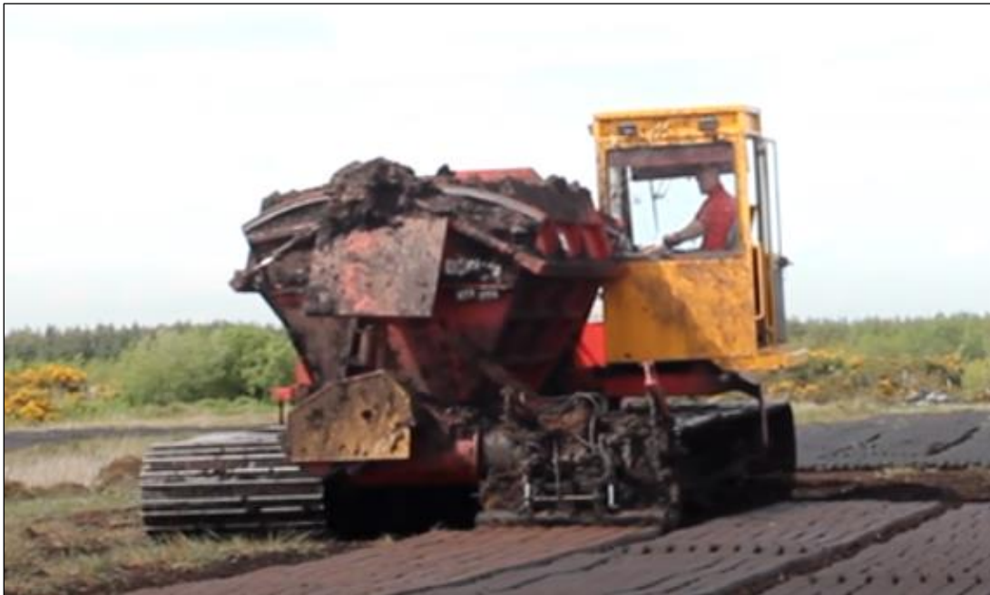
Plate 10-6: Difco Bogmiser Peat Hopper extruding rows of peat sods
