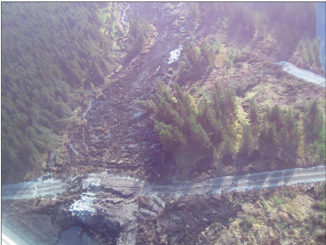
Plate 10-2: Aerial view of the head of the slide at Turbine T68 (October 2003)
