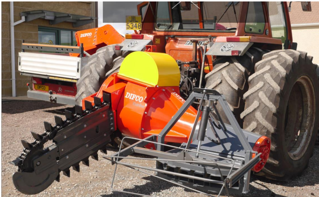
Plate 10-7: Typical saw cutting attachment for extracting peat
